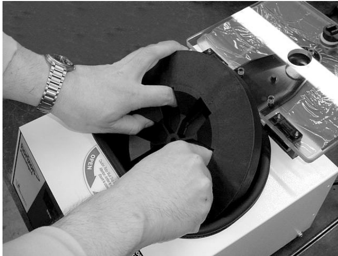
Proper position for removing or installing the performance-plus rotor
