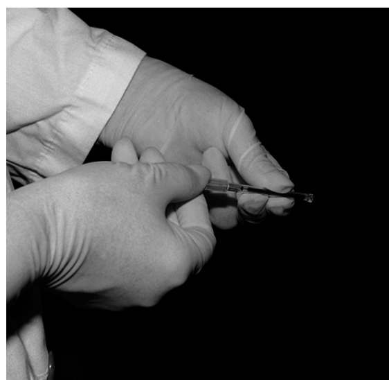
Figure 17 – Seating the Cap and Float
