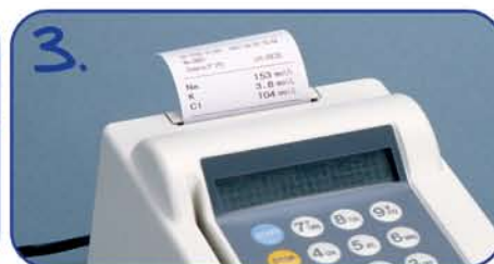
Remove pipette. Measurement starts automatically. Results in one minute
