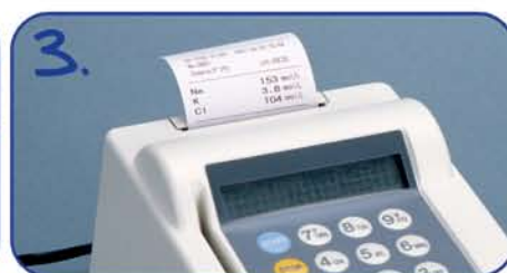
Remove pipette. Measurement starts automatically. Results in one minute
