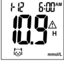
The display shows the number 10.9 in a large font, with mmol/L below it. To the right of the number is a triangle with an H inside (HI alarm icon). In the bottom left corner, there is a small icon of a cat's face.                              | $\triangle_H$ appears when the result is HIGHER than the “HI alarm setting” reference range. | For reference, or the default setting value can be changed 10.0 mmol/L (180 mg/dL) according to page 21. |
