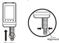
Insert the strip tray into the tray conveyor and the analyser will test automatically.
