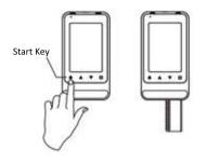
Press and hold the Start key for 3 seconds to turn the analyser on.
