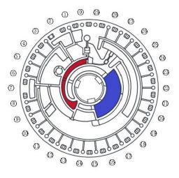
Each independently packaged reagent disc is formed by injection moulding a transparent material. A freeze-dried spherical biochemical detection reagent is arranged in the outer periphery of the rotor which is equivalent to a colorimetric device of a conventional biochemical analyser when the optical detection is performed. All blood separation, the mixing of the sample with the diluent and the biochemical reaction were performed on the reagent disc.
