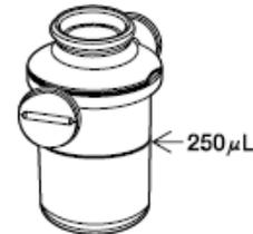
*Remove any air bubbles from the top of the sample prior to testing*
