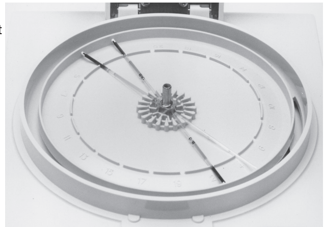
Figure 4-3. Typical Placement of Blood and Balance Tubes.
