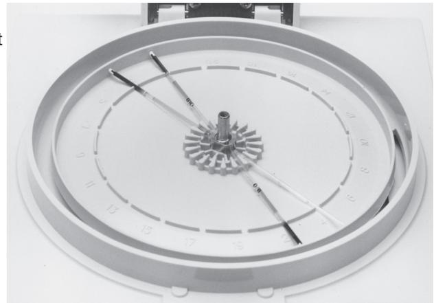
Figure 4-3. Typical Placement of Blood and Balance Tubes.
