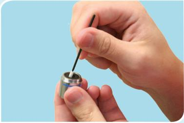
When performing internal cleaning, be careful not to press too hard against lenses and filters.
