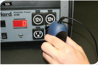
2. Using U.S.-style power adapter and power pack, plug ParaLens light source into portable power AC outlet.
