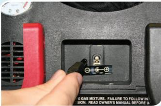
2. Insert Adapter plug into power input on back of Power Station.
