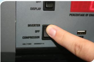
3. Toggle the inverter/compressor switch to the “INVERTER” position. You are now ready to power your ParaLens Advance LED light source.
