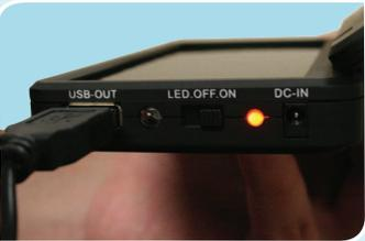
5. Turn power switch to “ON” position. If there is insufficient sunlight, indicator light will blink red.
