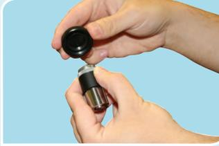
(Left) Unscrew main body assembly from protective casing cap by holding assembly and turning the cap in the direction shown.
