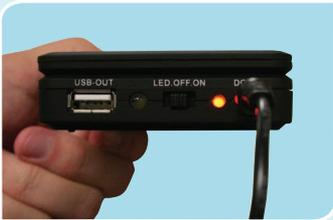
**3.** Plug DC wall adapter into solar pack “DC-IN” port and fully charge Li-ion battery. Red light indicates <50%, orange light indicates >50% and green indicates 100% charge.
