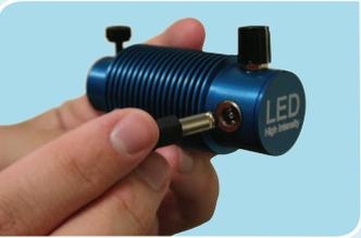
3. Plug large end of USB power cord into ParaLens Advance LED light source
