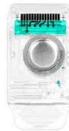
5-in-1 Cartridge Tests Electrolytes K + , Na + , Cl - , iCa 2+ & iMg 2+
