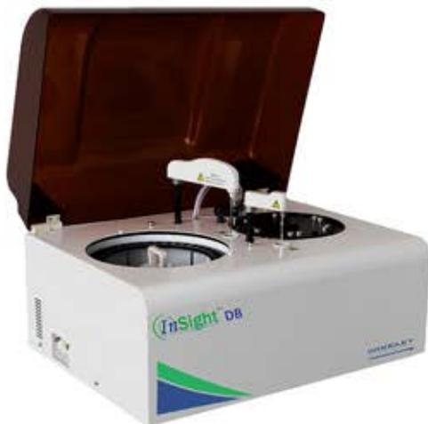
A fully automated clinical chemistry analyser which uses liquid reagents and is approximately 70% cheaper to run than dry chemistry
