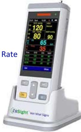
**Measure Blood Pressure, SpO<sub>2</sub>, Heart Rate, Temperature & Mean Arterial Pressure (MAP)**
