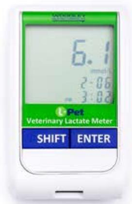
**An easy to use handheld meter providing blood lactate results in just 45 seconds**
