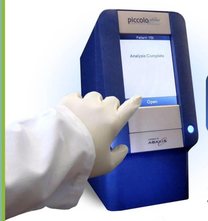
Press the Open button on the analyzer to open the drawer and discard the Disc.
